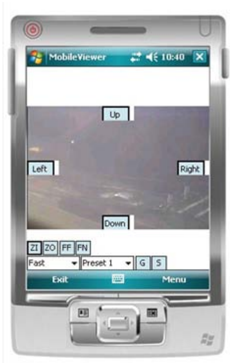
Figure 4.86. PTZF control screen
